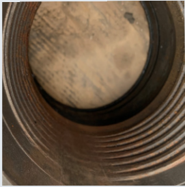
Type "H" BPV damaged during liner operations
